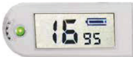
Figure 7. LCD showing an IOP measurement of 16 and statistical confidence indicator of 95
