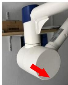
**Pull off the plastic cap at the rear joint of the spring arm.**
