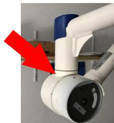
**View of the joint without plastic cap. The adjusting screw is positioned at the top.**
