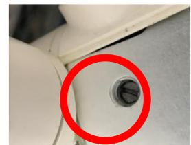
**Adjust the spring force with this screw according to the mounting instructions.**
